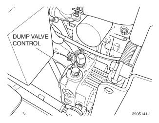
Figure 4-2. Dump Valve Control
